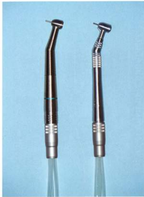
[Fig. 3] Handpieces tested left: new type handpiece with the Labyrinth right: conventional handpiece
